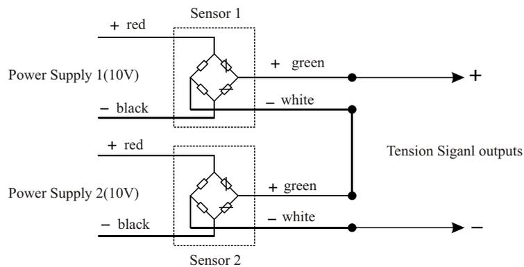
**Two tension sensor connection diagram**
