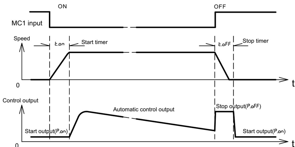
**Starting Procedure:** Before starting, TC950 outputs  $P_{on}$  to generate preparatory tension. When the Run/Stop switch (MC1-MCC) is turned on and after an overflow of time set in start timer  $t_{on}$ , the automatic control will start. At this time, indicator 'RUN' will be lit. See the figure above.
